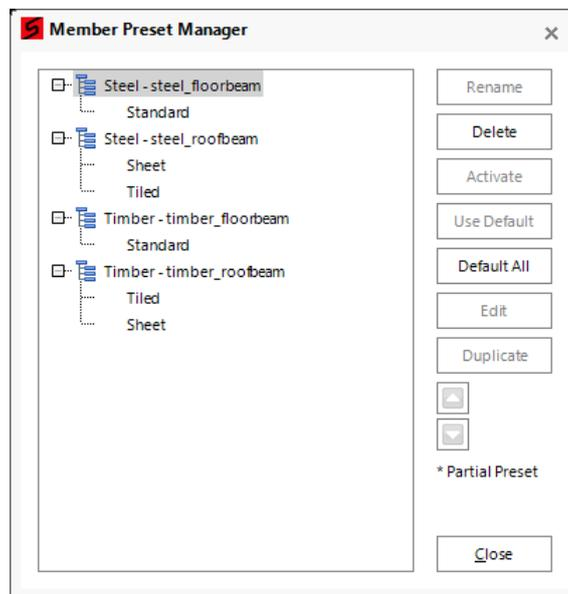
Within this interface, the desired presets can be activated for each module by either double-clicking or selecting it and pressing [Activate]. This will then show a green tick next to its name as seen below. Note the original default values can be used by pressing [Use Default] or [Default All]. Also note the selected preset will also persist to new projects until a different preset is selected.
